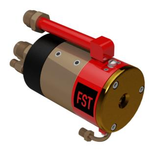
The SG-100 can use a variety of process gases including Argon, Nitrogen, Helium, and Hydrogen. When rebuilding is required, the SG-100's small number of components and selfaligning design make the job quick and accurate: the SG-100 cannot be assembled incorrectly and requires no adjustments.
